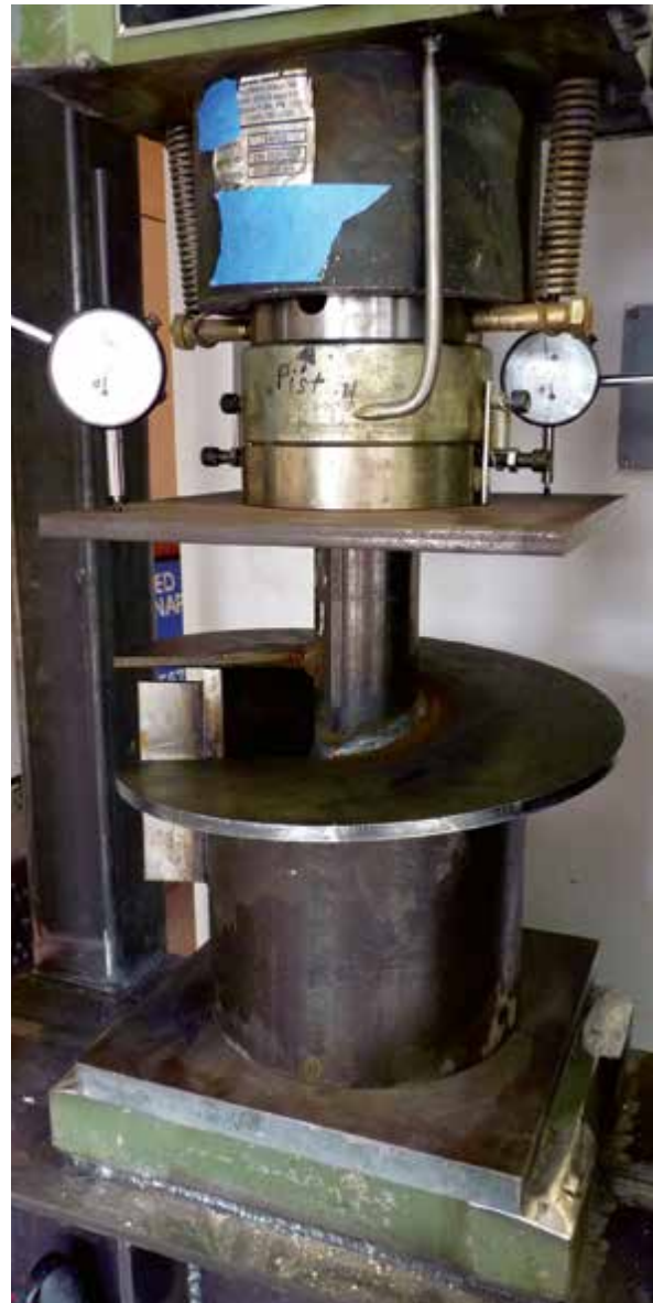
Figure 2A.1 Helix capacity testing of HP288 with 14-inch diameter helix plate
