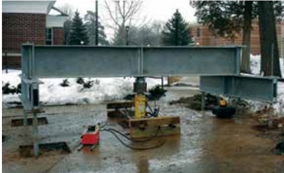
Figure 2.10.a1 Compression load test
