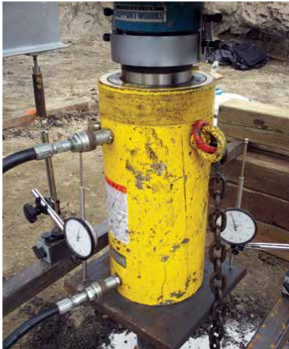
Figure 2.10.a2 Close up of test pile, hydraulic cylinder, dial gauges and hemispherical bearing plate
