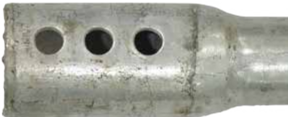
Figure 2.3.2.1.c Upset coupler with oversized closely-spaced bolt holes
