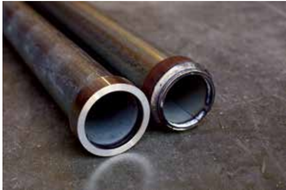
Figure 3.3.2.1.a PP288 starter tubes with pressed fit and welded friction reduction collars
