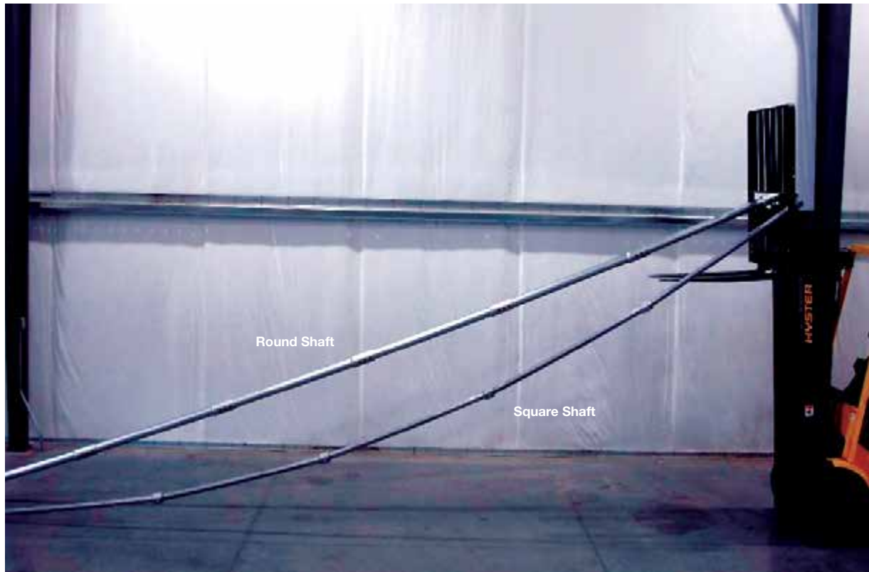
Figure 2.3.2.1.j Coupler Rigidity Comparison: FSI round shaft external welded coupler vs. typical upset coupler for square shaft
