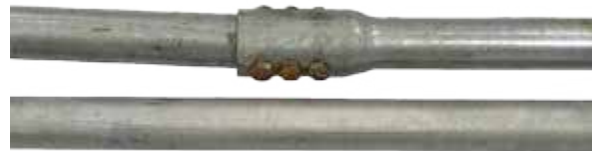
Figure 2.3.2.1.e Competitor upset coupler variance from straightness
