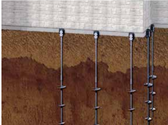
Figure 2.3.3.b1 Rendering of retrofit helical piers
