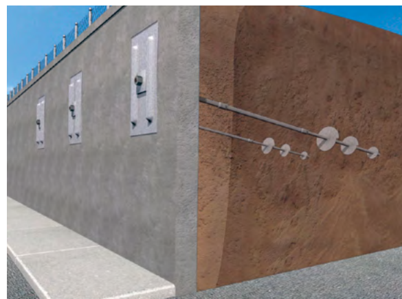
Figure 2.3.3.c Rendering of helical tieback installation
