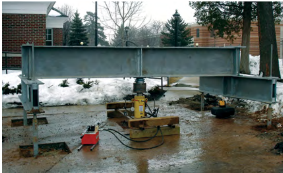
Figure 2.10.a1 Compression load test
