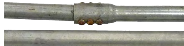
Figure 2.3.2.1.e Competitor upset coupler variance from straightness
