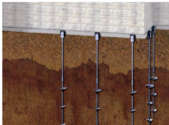
Figure 2.3.3.b1 Rendering of retrofit helical piers
