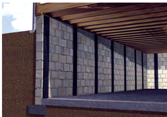
Rendering of the CarbonArmor® system installed within a basement
