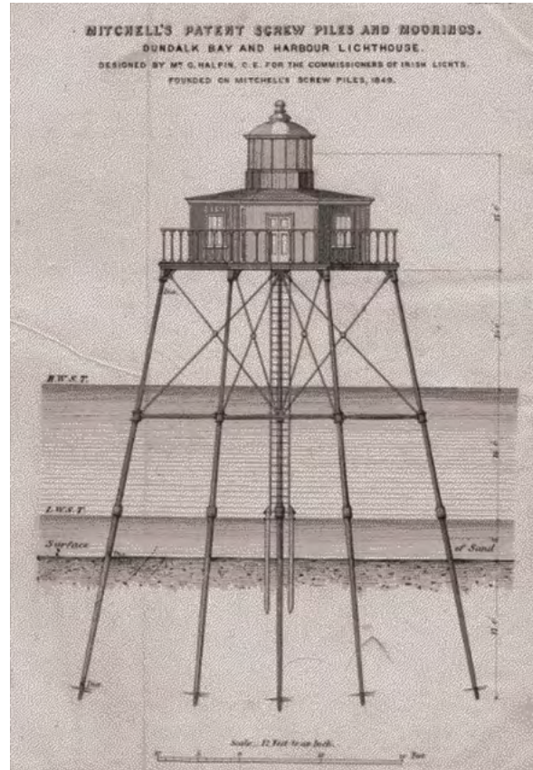
Early patent of screw (helical) piles
