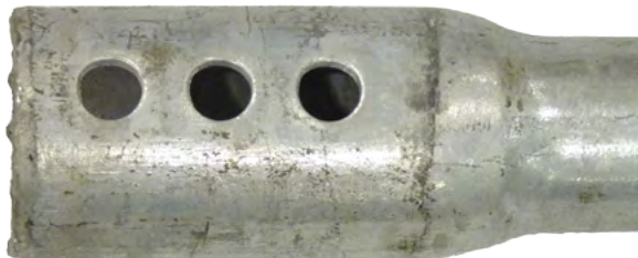
Figure 2.3.2.1.c Upset coupler with oversized closely-spaced bolt holes
