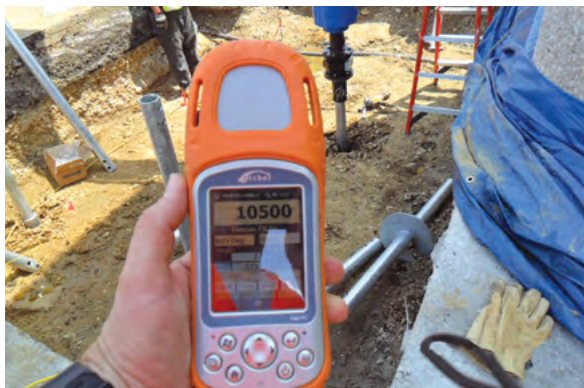
Figure 2.12.2.3.e2 Torque transducer providing direct reading of torque for helical pile project at Reagan National Airport
